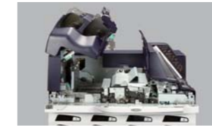
Removing jammed notes and foreign object from the counting section
